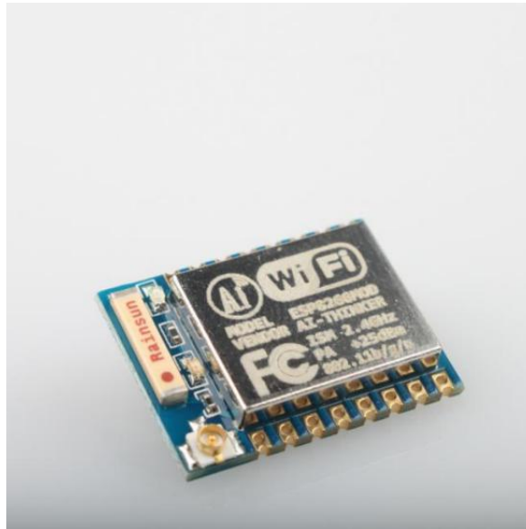
Figure 2 [Module Pin Counts, 16 pin, 16.0 mm x 21.2 mm x 3.0 mm]
