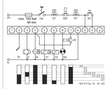
HS Mains switch GW Gas proving switch ST Limit thermostat RT
