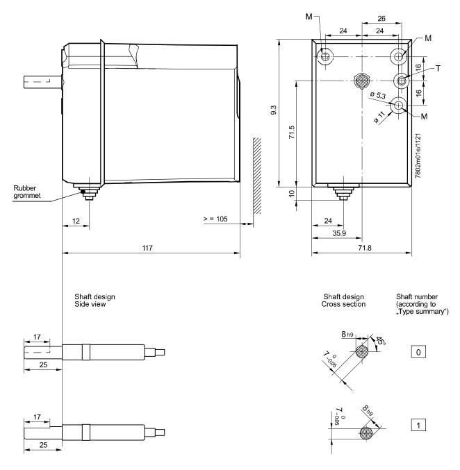
All shafts are shown in end switch position II CLOSED (as supplied).
