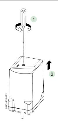
Step 3: Release the coupling while pressing the pressure pin down
